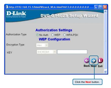
Enter the **Authorization Settings** you want to use for your WLAN network. Initially, you can accept the default value (**No Auth**) and change the router's configuration later. If you choose use Wireless encryption, click the **WEP** or **WPA-PSK** radio button to open the following screen.
